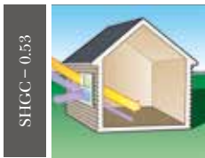
Standard clear unit, conventional aluminum spacer, air fill
